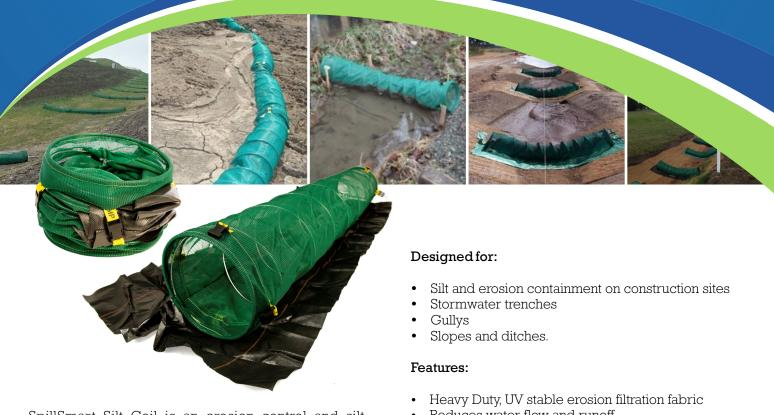
SpillSmart Silt Coil is an erosion control and silt management device designed for slopes, stormwater trenches, gully's and highway ditches. Its tubular fabric reduces the rapidity of water whilst capturing sediment, preventing harsh downstream erosion. Anchoring skirts secure the berm in place, whilst a spiral spring retains its cylindrical framework.
