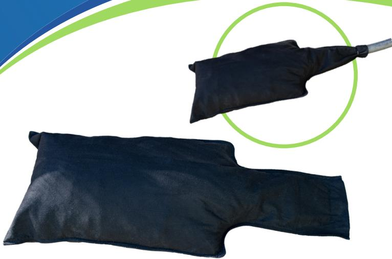
The SpillSmart Portable Oil and Water Separator acts as a disposable filter allowing untreated wastewater to pass through the filter bag whilst capturing sediment and hydrocarbons. These filter bags are filled with High quality shredded Oil Only, Melt Blown Polypropylene that successfully soaks up most of the oil passing through, before arriving to the 270gsm Geotextile outer lining.
