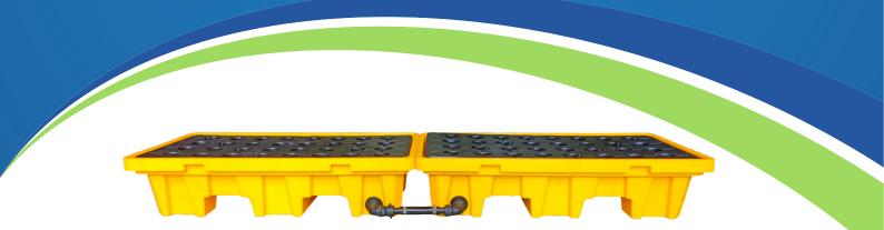
The 4 Drum Inline Bunded Pallet Set is sometimes referred to as a Bund Accumulation Centre. Each Bunded Spill Pallet is 1320mm x 680mm with a low profile of just 300mm. The two Pallet Bunds are secured into place with 8mm bolts end to end, with a Bridging Hose connecting into both Bund Sumps via two 32mm Nyglass Elbows. With the Bund Sumps now joined together the total capacity is now increased to 240L.
