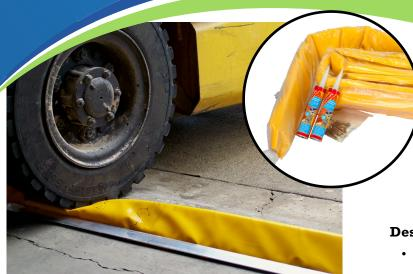
SpillSmart Drive Over Floor Bunding is designed for applications where non-aggressive liquids are being stored and where lower volume forklift or truck access is required. It's constructed with HF welded Heavy Duty 900gsm PVC, encasing high quality 100% memory foam. This combination provides durability and ease of access. The memory foam instantly returns to shape once clear of the vehicle's wheels.
